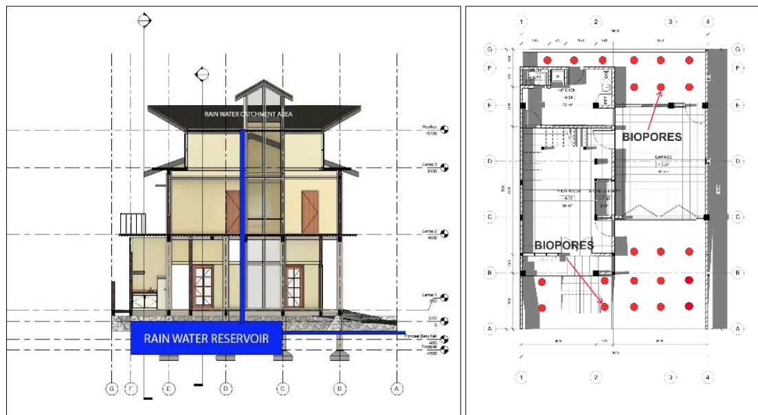
Figure 7 Rainwater Harvesting scheme and bio pores of Trisakti University, Nagrak campus's lecturer housing
