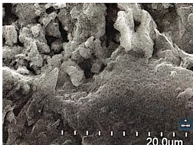
Fig. 9. SEM Analysis of Dried AgNPs at 20,000x Magnification.
