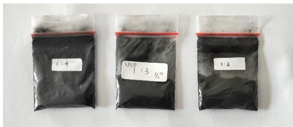
FIGURE 1. Powders of Perovskite Oxide of \text{La}_{0.7}\text{Sr}_{0.3}\text{CoO}_{3-\delta}
