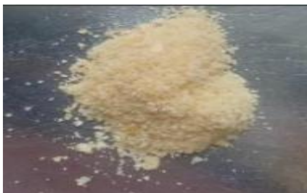
Figure 1. Milkfish bone gelatin: Gelatin obtained from the milkfish bone synthesis process using 5% phosphoric acid solution ( H_3PO_4 )
