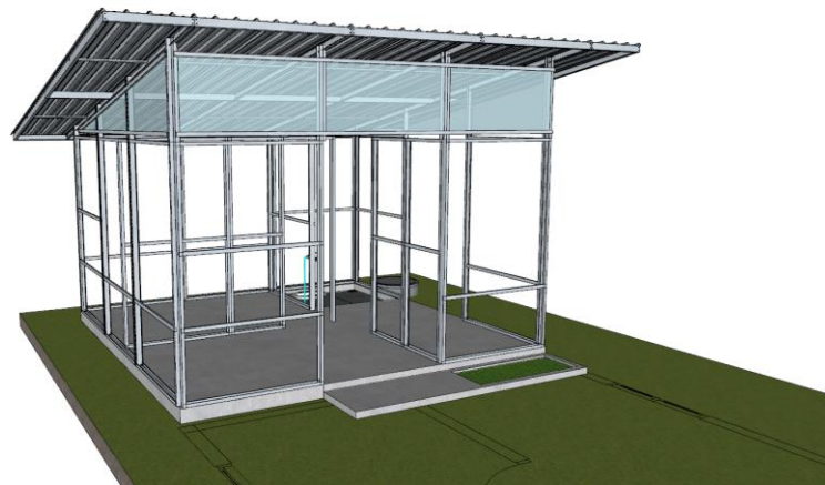
Figure 3. The structure plan of temporary housing
